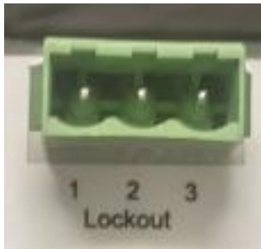
Figure 8-1 charger lockout relay terminals. 1=NC, 2=COM, 3=NO
